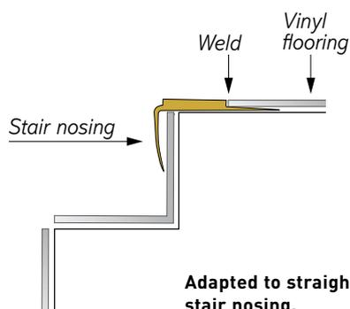
Adapted to straight stair nosing and rounded stair nosing.
