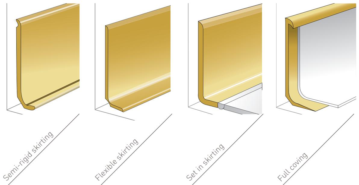
**There are two ways of finishing the junction between the floor and wall:**
